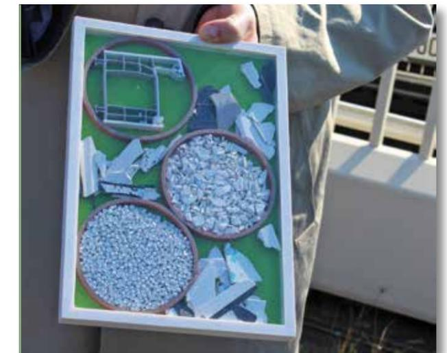
Display for the mechanical recycling of PVC window frame
