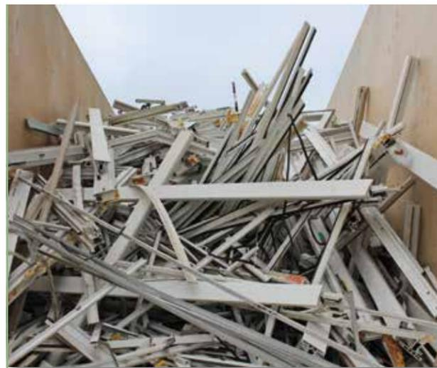
Raw material for new recycled window frame profiles
