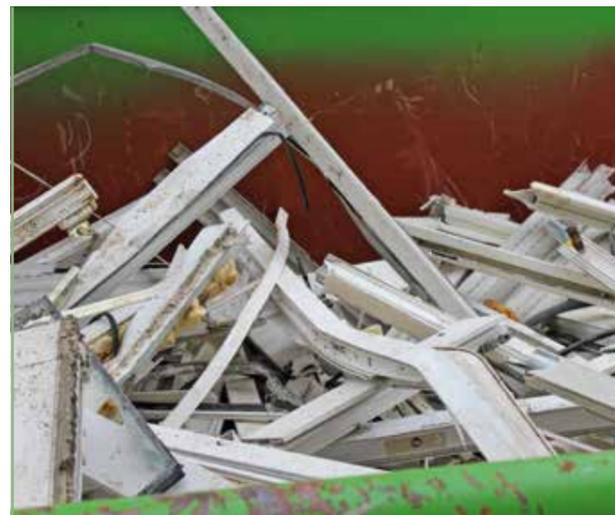
Used PVC window frame profiles for material recycling
